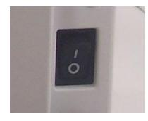
Turns the sewing machine on or off.
