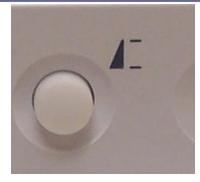
Stops the machine at the end of a single stitch or stitch combination.
